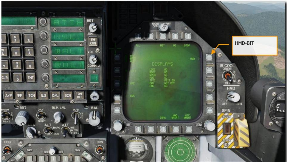
Abbildung 160. HMD Built in Test (BIT)160
